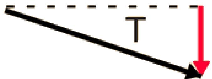
For the same internal pressure, the downward component of the tension must be the same.
